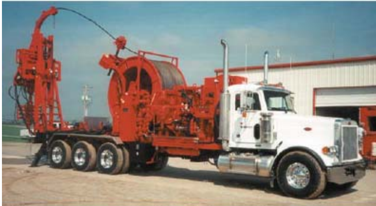
Figure 7 Truck Mounted Winch and Injector System
