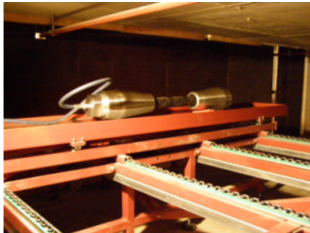
Figure 5: Airborne's in-house pressure test facility
